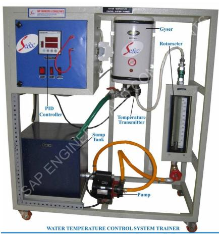
The Water Temperature Control Trainer (PCST - 08) is the system, which outlines the basics of Closed Loop Water Temperature Control and various aspects related to it. KEY WORDS:
